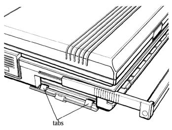
11. Lift the cover up into place and slide the release tab up to secure the cover.
